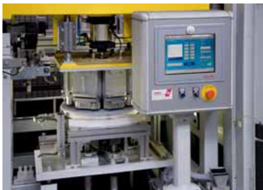
The three individual parts are welded at eleven points to form a complete assembly
