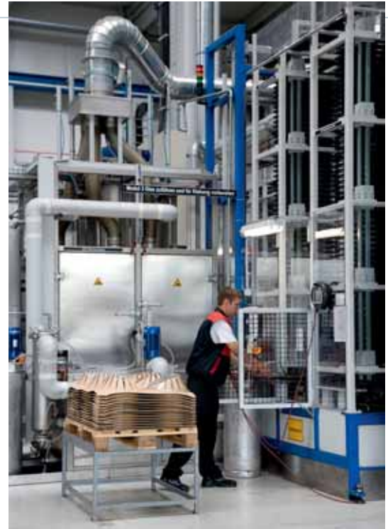
The glass doors are loaded onto the production line manually. The glass door washing unit and buffer store can be seen in the background
